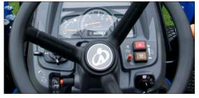
Easy to read electronically operated dashboard with rev counter, fuel gauge, PTO controls and light switches.
